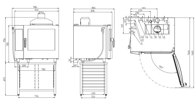
${f A}$  - Flap valve,  ${f B}$  - Chimney,  ${f C}$  - Drain,  ${f E}$  - Electricity,  ${f G}$  - Gas,  ${f V1}$  - Untreated water,  ${f V2}$  - Treated water
