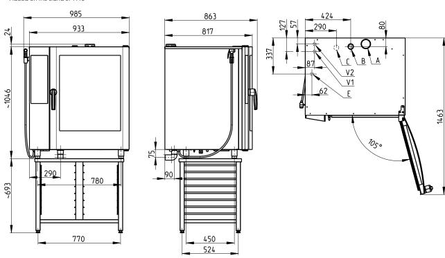
A - Flap valve, B - Chimney, C - Drain, E - Electricity, V1 - Untreated water, V2 - Treated water
