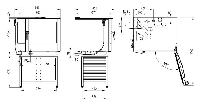
A - Flap valve, B - Chimney, C - Drain, E - Electricity, V1 - Untreated water, V2 - Treated water
